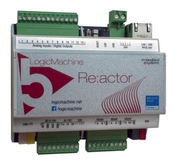
with cloud/web services, 3<sup>rd</sup> party devices. Via applying custom scripts LM can simultaneously act as thermostat, security panel, lighting controller, etc. LogicMachine application store and external app development possibility allows to extend device functionality and adjust to a specific market segment.
