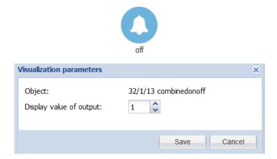
• *Display value of output* - selects which object number (1..16) is used for value display
