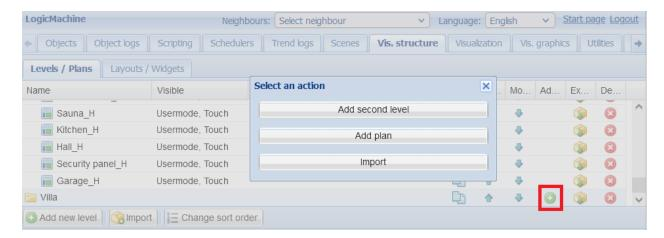
Select *Import* to import levels and plans from a file (it can be exported from another LM). Object links between visualization elements and group addresses can either be cleared or kept.
