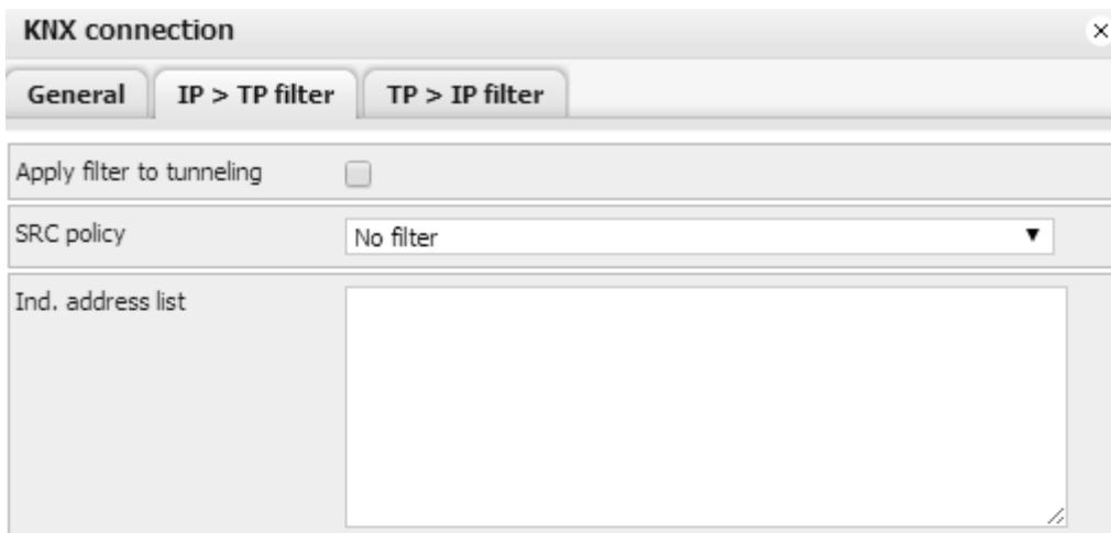
**Info:** One address/range per line. Use \* (e.g. 1.1.\* ) to filter all addresses in the given line.
