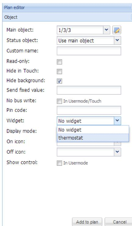
Once added, you can try out the widget in *Usermode visualization* by clicking on added object (temperature sensor icon on the left), the widget appears on click.
