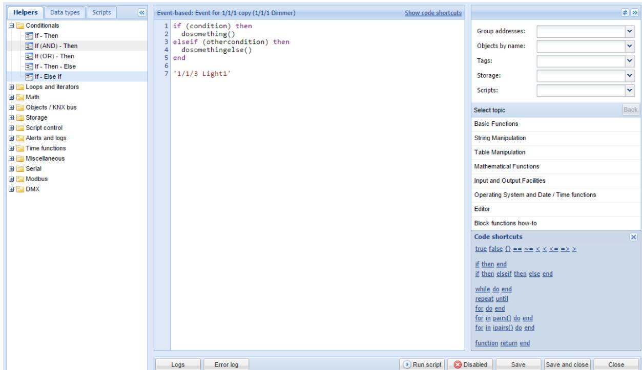
There is also a code shortcut button, which helps with most common function structure.
