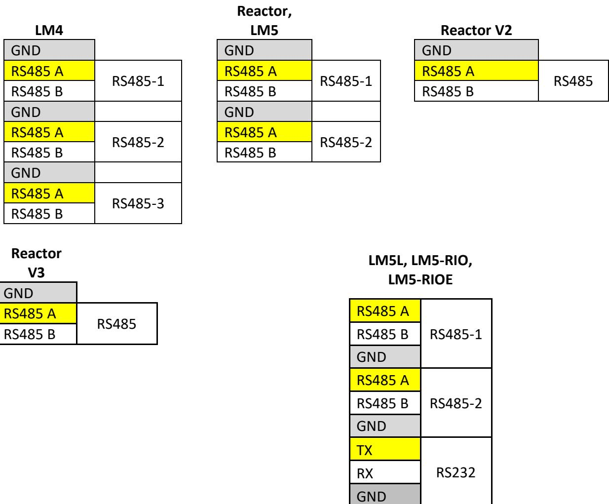
Note! LM5 series devices have 1 definitive serial port RS-485 and other one can work either as RS-485 or RS-232. The one will work which is most recently opened.
