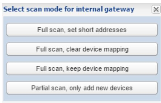
**Full scan, set short addresses** - scans for currently connected DALI devices to the selected gateway, assigns short address automatically starting from 0,1,2,...
