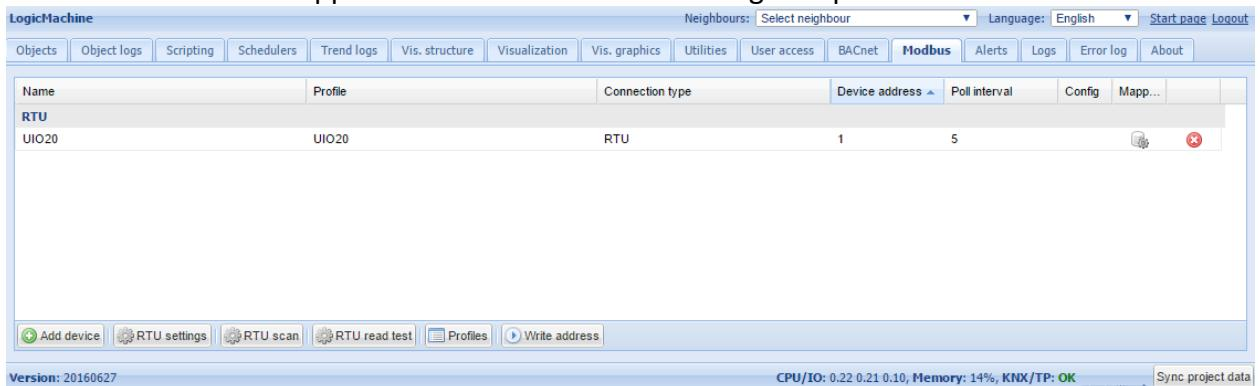
**Modbus Master** – user graphical mapper interface in Modbus tab
