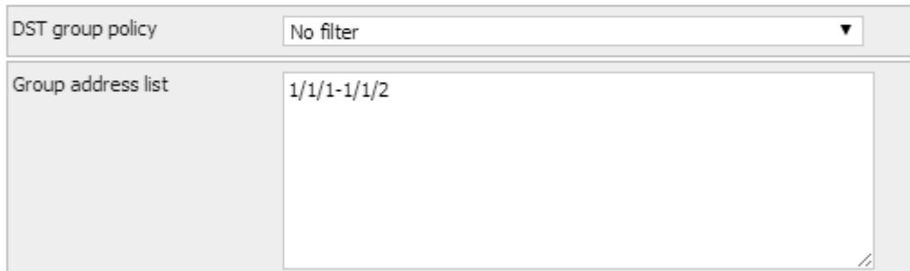
**Info:** One address/range per line. Use \* (e.g. 1/1/\*) to filter all addresses in the given line.
