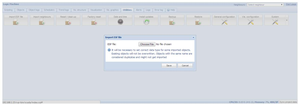
Or connect LM to the bus and it will detect objects automatically (in yellow) in *Objects* tab once they are activated. Objects can be added manually as well.
