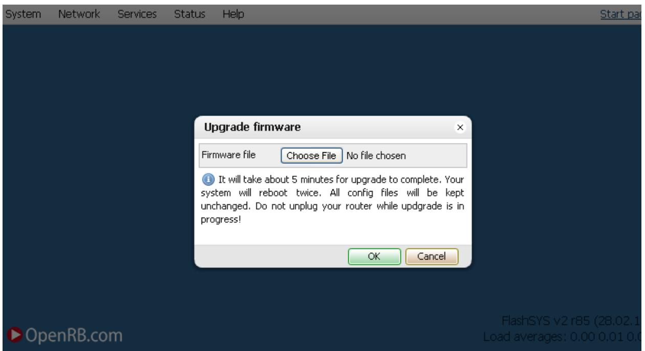
LogicMachine visualization upgrade or patch installation can be done in *Utilities* tab and press on *Install updates* icon. After \*.LMU file is chosen from the corresponding location press *Save* button. The device will be rebooted after 5 seconds and new firmware will be installed.
