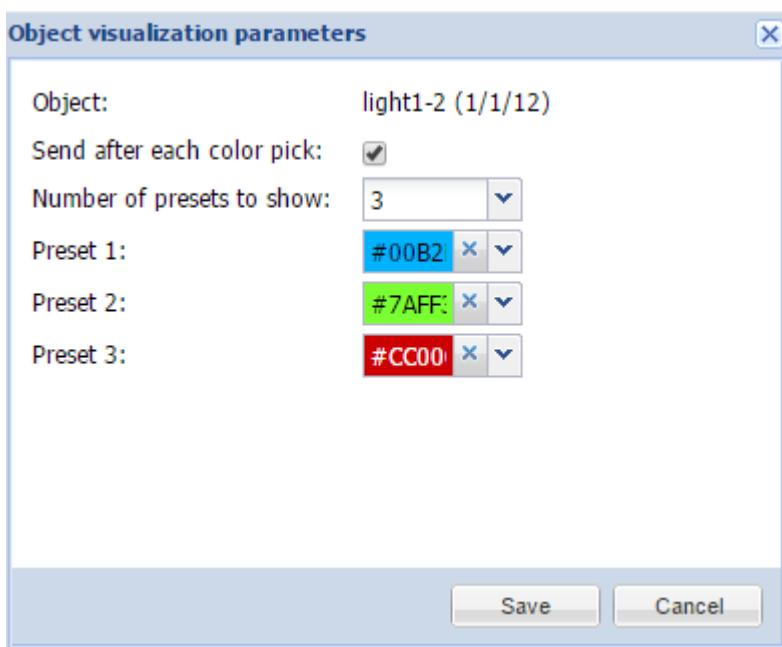
**Send after each color pick** – specifies either to send the telegram automatically into KNX bus once the color is selected in color picker.
