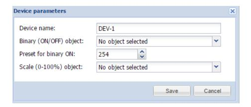
**Device name** – name of the DALI device **Binary (ON/OFF) object** – map to KNX binary object **Preset for binary ON** – preset on binary ON **Scale (0-100%) object** – map to KNX scale object
