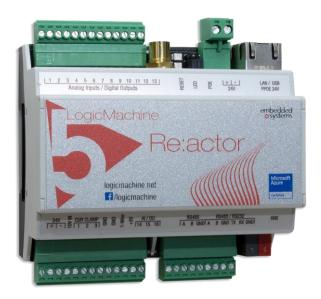
applying custom scripts LM can simultaneously act as thermostat, security panel, lighting controller, etc. LogicMachine application store and external app development possibility allows to extend device functionality and adjust to a specific market segment.
