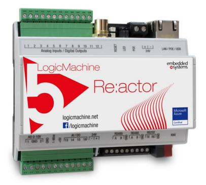
interface and integration with cloud/web services, 3<sup>rd</sup> party devices. Via applying custom scripts LM can simultaneously act as thermostat, security panel, lighting controller, etc. LogicMachine application store and external app development possibility allows to extend device functionality and adjust to a specific market segment.
