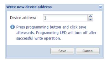
There is a separate Write address button to program address for UIO20 device. Press programming button and click save afterwards. Programming LED will turn off after successful write operation.
