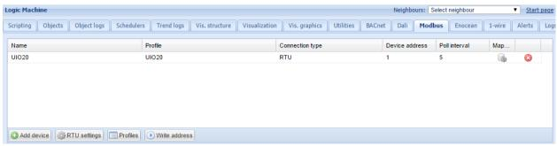
Modbus Master – user graphical mapper interface in Modbus tab
