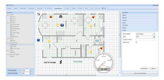
Once the gauge parameters are defined, press *Add to plan* button and newly created object will appear on the map. You can move the object to the location it will be located. Press on *Save and reload plan* button so the objects starts functioning.
