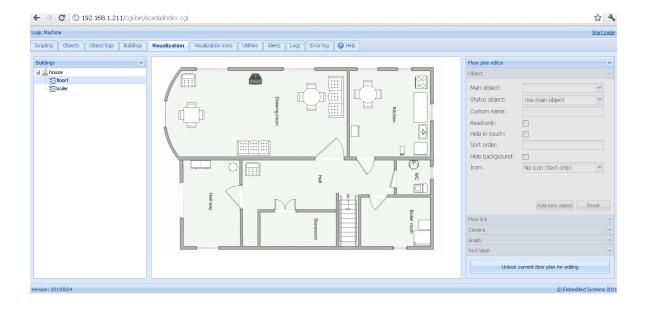
Existing objects can be added to the map by clicking on *Unlock current floor plan for editing* button. Once the object parameters are defined, press *Add new object* button and newly created object will appear. You can move the object to the location it will be located. Note that while being in editing mode, the object will not work.
